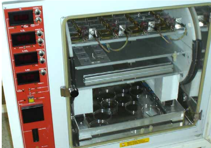
Figure 2 Adapted Heraeus Cytoperm incubator for incubating organotypic cultures. The shown incubator was adapted by the user for culturing organotypic slices on MEAs. It is possible to incubate the MEAs only and remove them from the incubator for recording, or to incubate complete MEA1060 amplifiers (see top shelf) and record inside the incubator.
